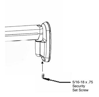
Figure 7. Install Security Set Screws (Option II)
